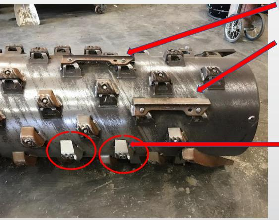
Location of the Straight Separator bars, leading into each other. Total of four is used. p/n-1318976C2
