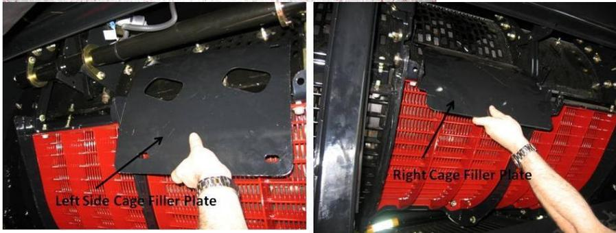
Location for filler cage plates would go above the #2 Module section.
