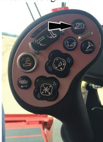
5) The Automation can be fine-tuned if need be. Use the funnels to change the sensitivities. Also, refer to the operator’s manual for further explanations of the sensitivities.
