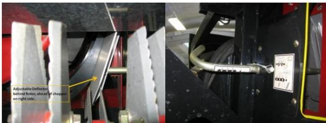
**-10/20/230 Series Combine Residue kits-** Part # is **51474747**. This is latest divider currently used on 250 Series. Provides a better residue spread.
