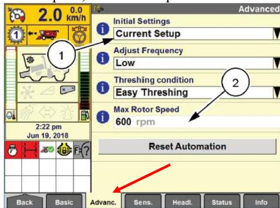
4) Use the Feed rate, be sure to use this mode when using the Automation. Sometimes this is called “Cruise Control” which allows the Combine to vary the ground speed automatically while optimizing the settings.
